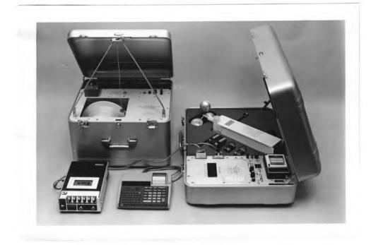
Figure 12. Tethersonde equipment. Left rear-electric winch. Left to right, foreground-cassette recorder, Hewlett-Packard HP-97 Programmable Printer/Calculator, ground station with airborne package.
