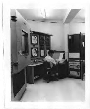
Figure 72. NCAR Computer-Controlled Environmental Chamber. The one-cubic-meter chamber is on the left and the computer controller is on the right. Photo courtesy of NCAR.
