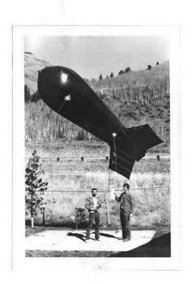
Figure 11. Normal operating configuration of tethersonde balloon and airborne package.
