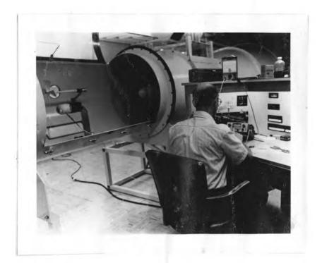
Figure 71. Closeup of test section of NCAR Wind Tunnel. Control panels are on the operator's console at right. Photo courtesy of NCAR.
